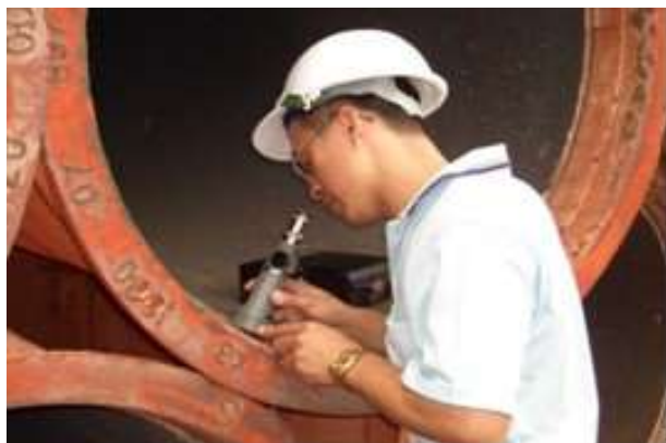
Pipe inspection on piping factory
